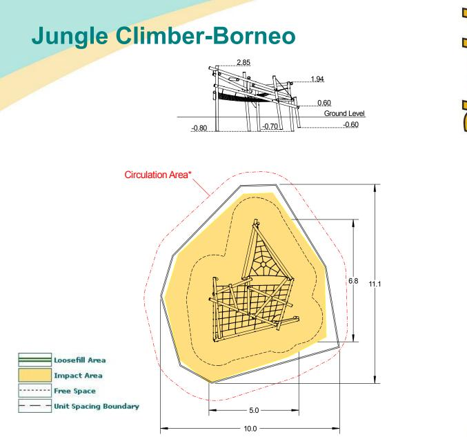
\* Recommended Circulation Area (1.2m outside impact area) – this area should be clear of solid raised objects (ie fences, walls, trees and other items of equipment). Loose fill retaining edgings are acceptable in this area.
